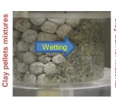
Homogenized clay barrier material
